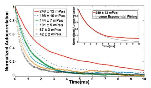
FIG. 2. (Color online) Representative  $g_{HV}^{(1)}(\tau)$  for samples with varying viscosity. Decay time is observed to decrease as the viscosity decreases. The inset shows a representative inverse exponential fitting to  $g_{HV}^{(1)}(\tau)$  (dotted line), based on Eq. (1).
