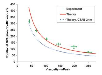
FIG. 3. (Color online) Comparison of experimental  $D_R$  with theoretical predictions assuming GNRs as smooth cylinders [14] (solid line: for the actual sizes of the GNRs; dotted line: considering an average CTAB layer of 2 nm).
