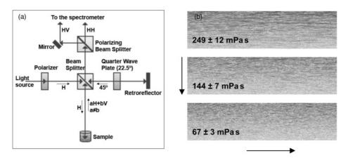
FIG. 1. (a) PS-OCT interferometer setup. (b) Example *M*-mode images [using an absolute value of  $\tilde{a}(z,t)$ ] in the *HV* configuration showing an increasing rate of intensity fluctuations for samples with decreasing viscosities. (Note: Intensity fluctuations only up to 40 ms shown.)
