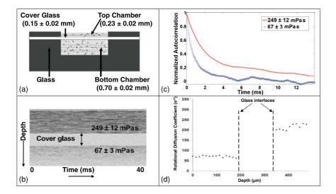
FIG. 4. (Color online) (a) Doublechamber design. (b) *M*-mode images [using an absolute value of  $\tilde{a}(z,t)$ ] showing samples with different viscosities separated by a cover glass. (Note: Intensity fluctuations only up to 40 ms shown.) (c)  $g_{HV}^{(1)}(\tau)$  of the samples showing two different decay time scales. (d)  $D_R$  as a function of depth in the double chamber.
