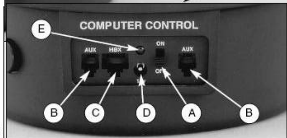
Fig. 2 (Inset): Computer Control Panel. (A) On/Off switch; (B) Auxiliary ports; (C) Handbox port; (D) 12v connector; (E)
