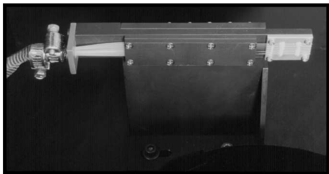
FIG. 3.—Fiber output assembly. Three pairs of fibers with diameters of 100, 200, and 300 \mu\text{m} are arranged vertically, with the smallest fibers at the center and the largest fibers at the top and bottom. The ends of the fibers are aligned precisely in six V-grooves; the V-grooves are bead blasted but not anodized (see § 3.4).
